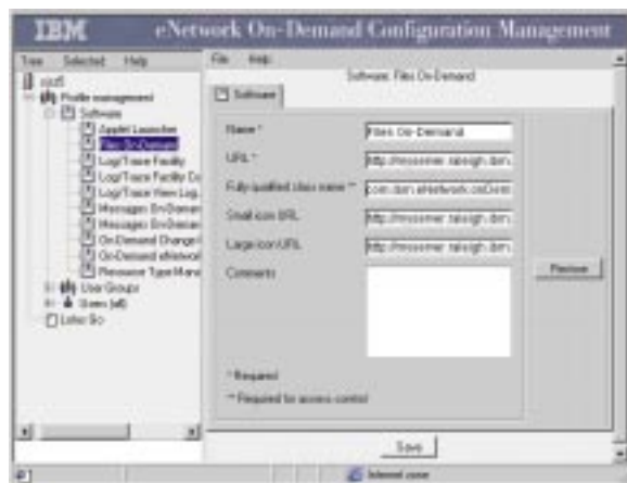
Figure 2: Your favorite Web browser is all you need to run On-Demand's Profile Manager
